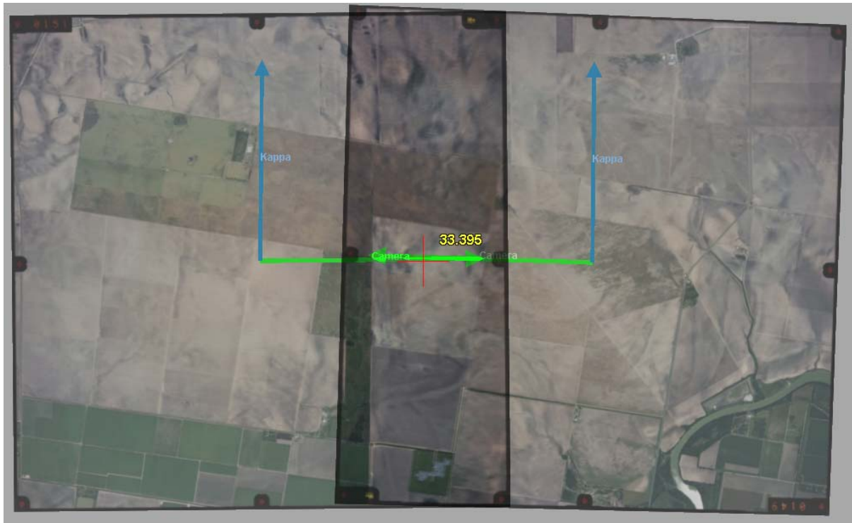
Camera direction and kappa angle display for two end-overlapped images from different strips. The camera angles are opposite each other, since the airplane was flying different directions for each image. The origin for each arrow set is at the image center. Zoom out if this is not currently visible.
